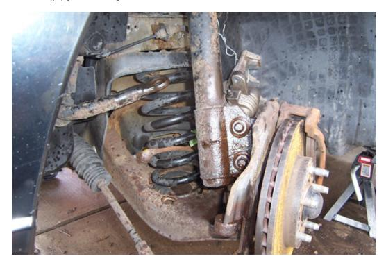
5. Carefully remove the three strut-to-body mounting nuts/bolt. When these are detached, the strut is free to drop out, so use one hand to cushion its fall so that it does not damage any front end parts. Keep the square mounting plate from the strut-to-body nuts/bolt and reuse.
