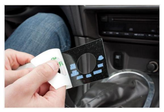
3. Only one side will fit in at a time. Start by sliding the top of the gauge face up into the bezel far enough that the bottom of the face will clear the bottom of the bezel. Then line up the holes and press firmly to adhere.
